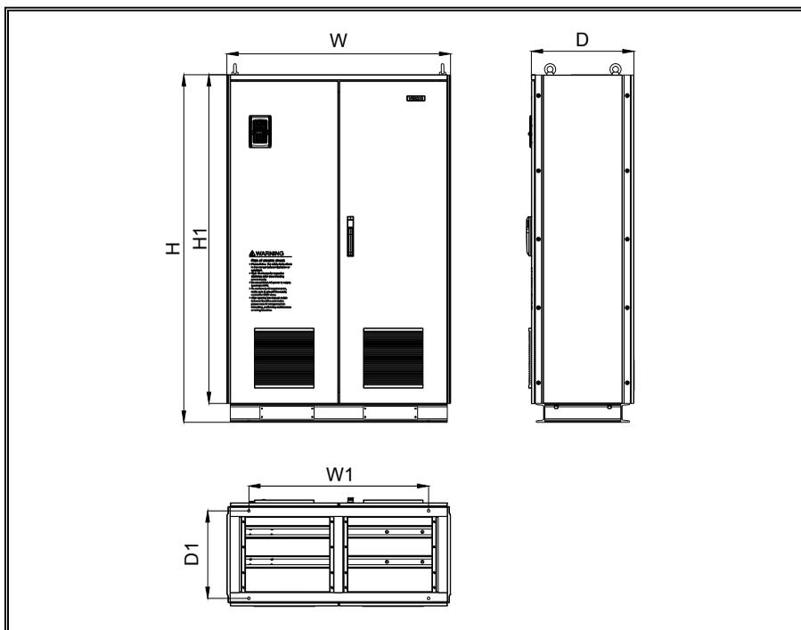
The technical drawing illustrates the AC100 series inverter cabinet from three perspectives: front, side, and top. The front view shows a cabinet with a width dimension  $W$  and a total height dimension  $H$ . A specific height dimension  $H1$  is also indicated. The side view shows a depth dimension  $D$ . The top view shows a width dimension  $W1$  and a depth dimension  $D1$ . The front view also includes a warning label and a handle on the right door.
